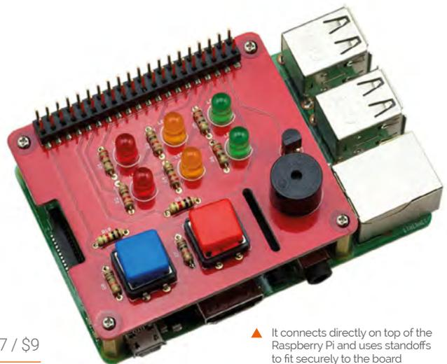
▲ It connects directly on top of the Raspberry Pi and uses standoffs to fit securely to the board
