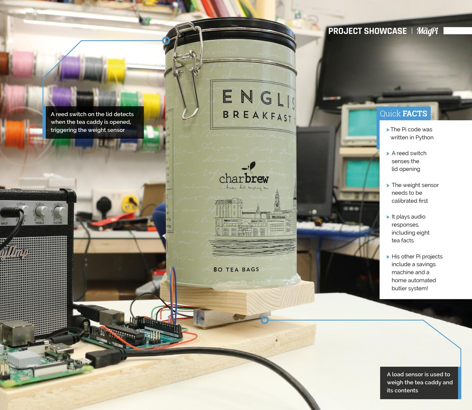
A reed switch on the lid detects when the tea caddy is opened, triggering the weight sensor
