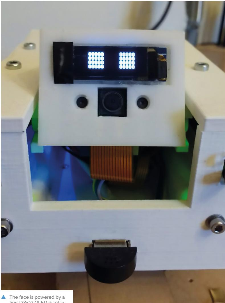
▲ The face is powered by a tiny 128x32 OLED display
