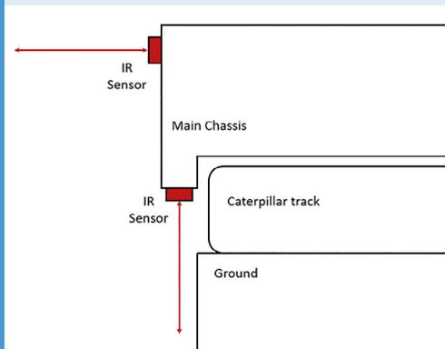
**02** The Raspberry Pi is constantly monitoring the IR sensors via the GPIO header, and runs the results via the software.
