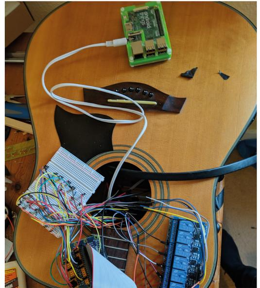
▲ The Pi and other components, including an eight-channel relay for the solenoids in the Braille reader, are stuffed inside the body of the guitar
