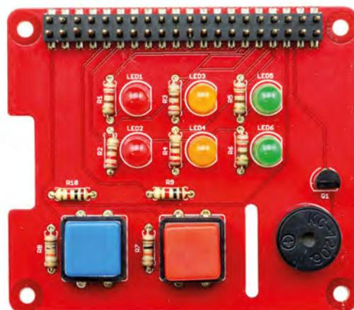
▲ The JAM HAT adds six LED lights, two buttons, and a buzzer to the Raspberry Pi
