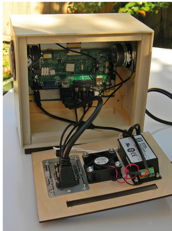
▲ Cables run from the circuit board of the monitor to the back of the new case, so that the connectors are easily accessible. Components are cooled by a fan
