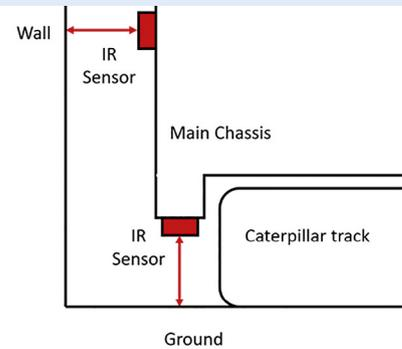
**01** The infrared sensors at the front detect a surface, or the IR sensors on the bottom detect a lack of a surface, so there is either a wall or a cliff in the robot’s path.
