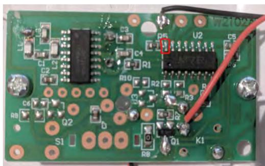
▲ Connecting the door-bell wiring to the Pi's GPIO pins
