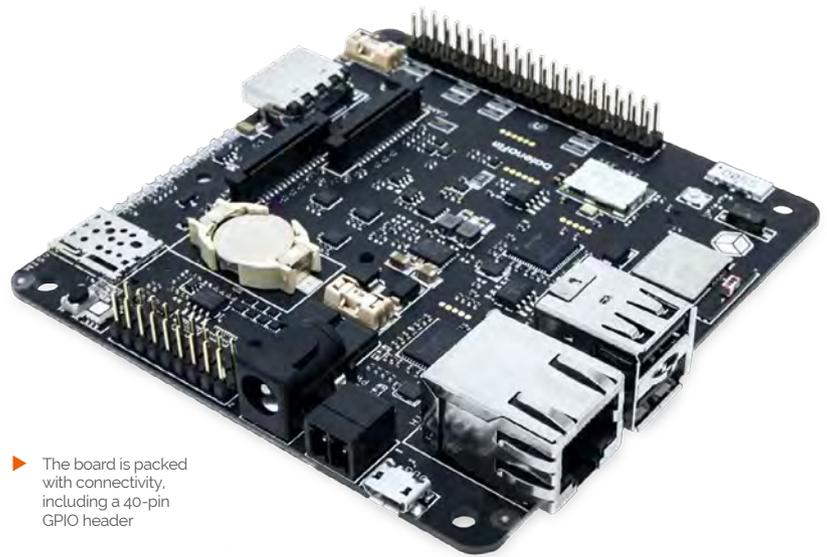
▶ The board is packed with connectivity, including a 40-pin GPIO header
