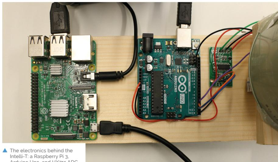
▲ The electronics behind the Intelli-T: a Raspberry Pi 3, Arduino Uno, and HX711 ADC
