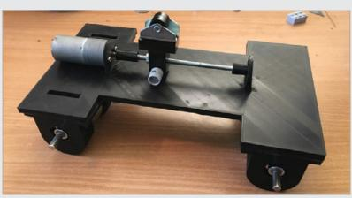
Above A long threaded bar converts motor rotation into lateral movement to tilt the whole firing mechanism (not shown) up or down for aiming purposes
