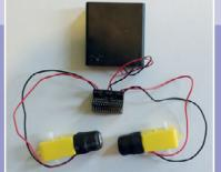
If your left and right are mixed up you can swap wires on the motor control unit or change GPIO values in the **robot** variable:
