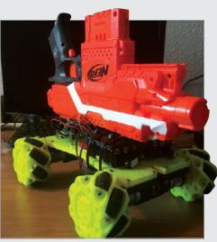
Continuing work on the project, David plans to power it with LiPo batteries – "It currently runs on 14 (!) AA batteries which really don't last very long as the drive motors and flywheel motors are pretty greedy."
