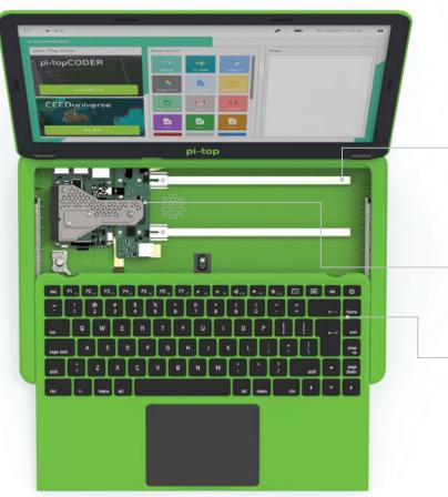
Two magnetic rails are used to quickly connect and remove components to the kit
