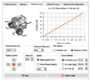
Above The Vehicle Control panel provides options for driving by distance, angle, and time, and can plot the resulting data
