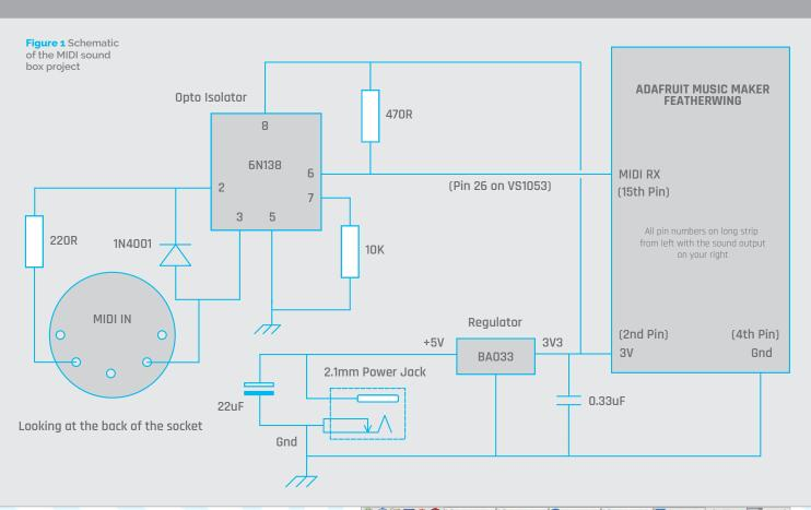
round), and also a current-limiting resistor for the LED inside the optical isolator. On the output side, a Darlington transistor pair picks up the infrared light from the LED and amplifies it. This signal can then be sent to the MIDI input of the VS1053. We need to feed the board with 3V3, so we have included a voltage regulator to do this.
