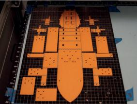
> STEP-03 Ready for assembly The shapes of the individual parts are cut from the laminated sheet. The holes are mounting holes, designed to be used with rivets.
