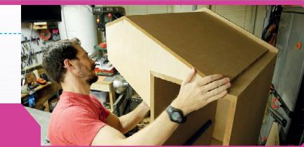
Bob cut a panel for the back cover and laid it over the top it's not nailed down, so you can quickly access the inside of the top sections.
