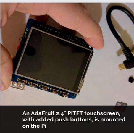
An AdaFruit 2.4" PiTFT touchscreen, with added push buttons, is mounted on the Pi
