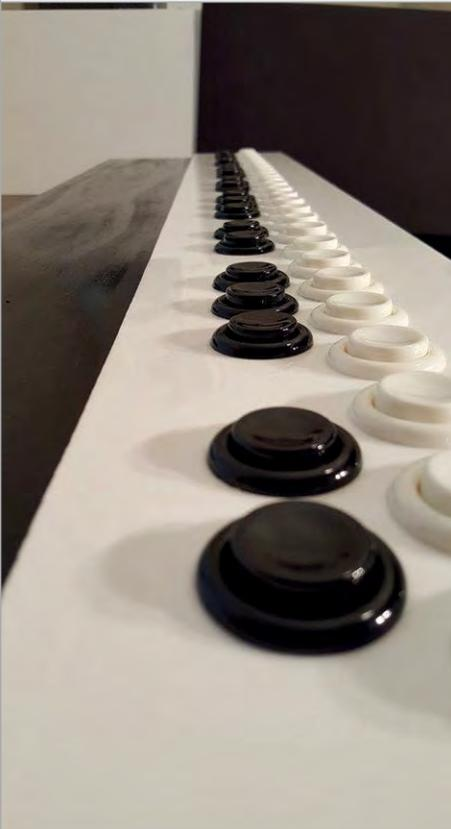
on the keys so they were, of course, prone to floating. At that point, I had inadvertently built a touchless piano,” recalls Brian. 1K resistors were added to each input to solve the problem. “There is still some noise on the audio despite using a clean power supply and line filter. Maybe using \$0.99 USB audio cards is to blame.”
