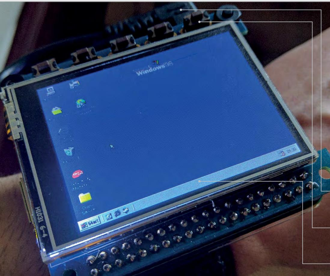
• A LiPo battery, hidden underneath, powers the Raspberry Pi A+ and touchscreen
