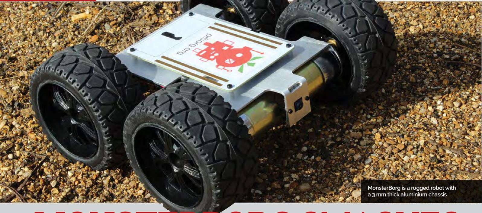
MonsterBorg is a rugged robot with a 3 mm thick aluminium chassis
