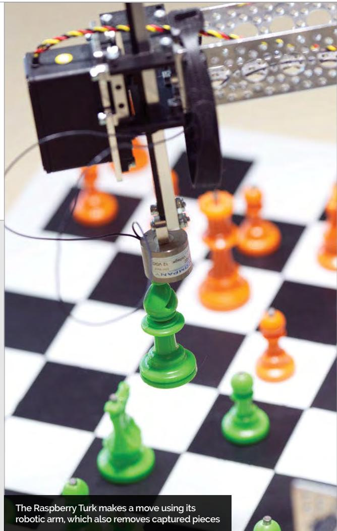
The Raspberry Turk makes a move using its robotic arm, which also removes captured pieces
