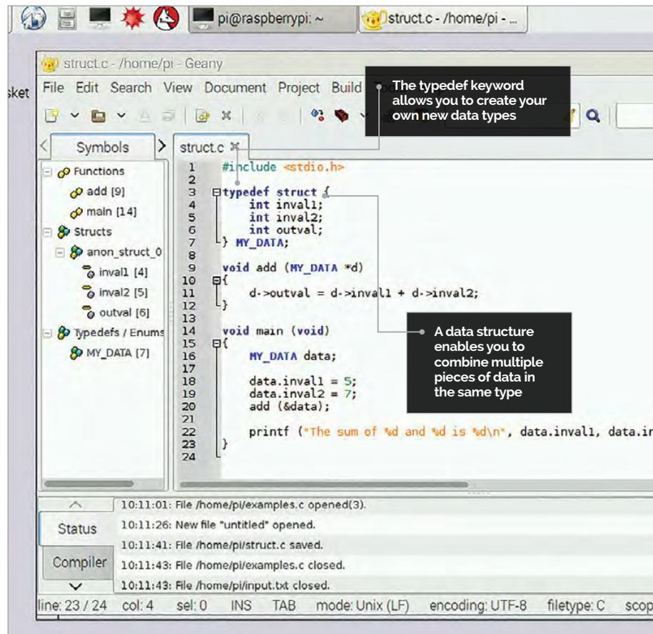
We use a typedef to create a data type called **MY\_DATA**. The definition of the structure consists of the keyword **struct** with a list of variables enclosed by curly brackets. In this case the structure consists of three integer variables.
