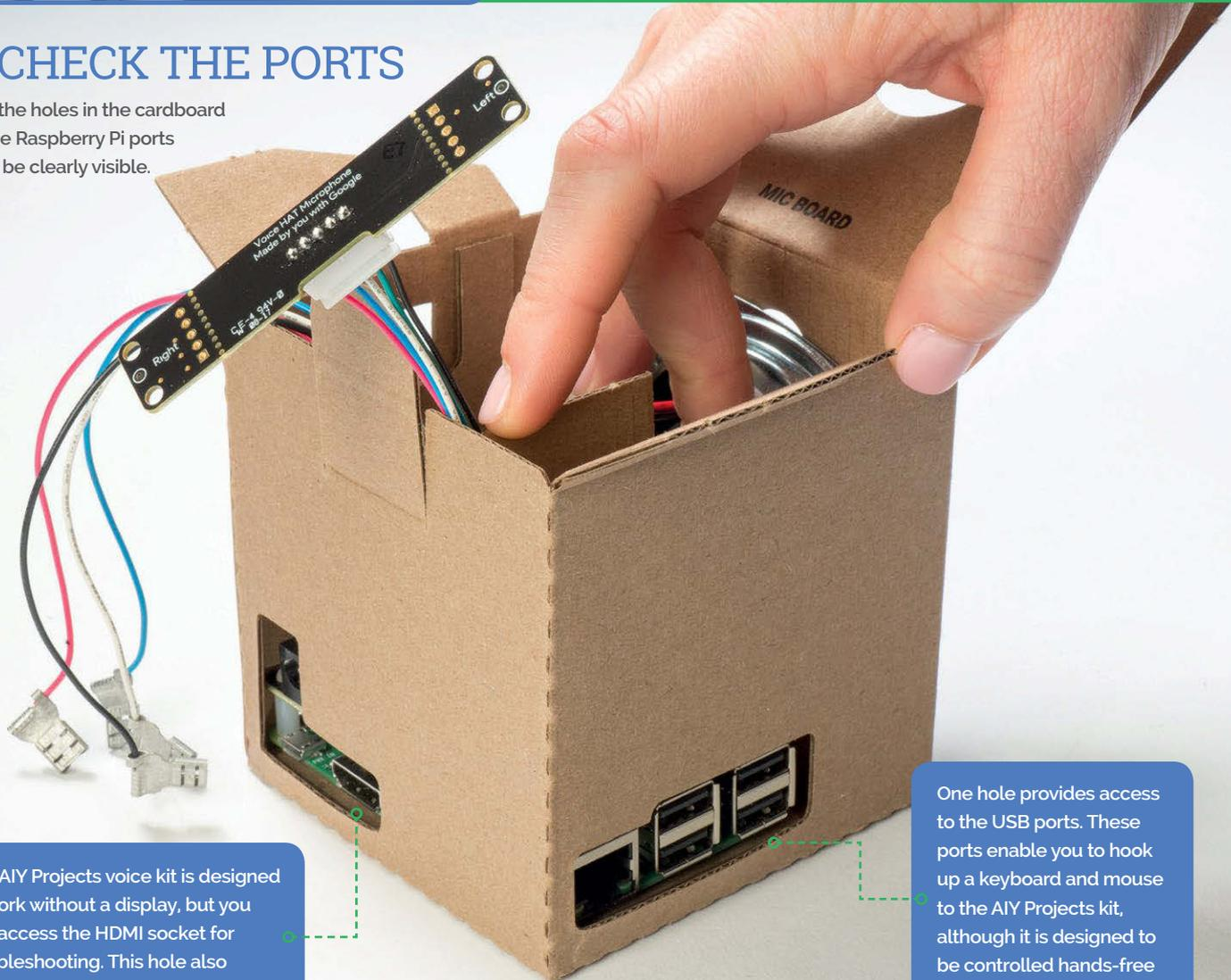
The AIY Projects voice kit is designed to work without a display, but you can access the HDMI socket for troubleshooting. This hole also provides access to the power socket.
