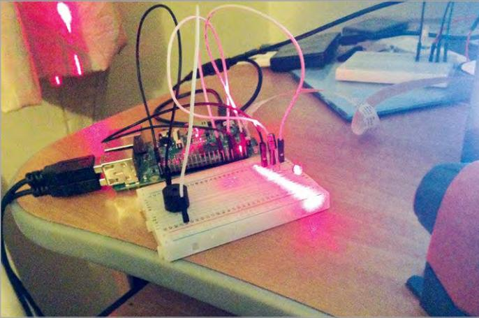
**Above** Shining the laser onto the LDR in a darkened room will dramatically affect the measured light level
