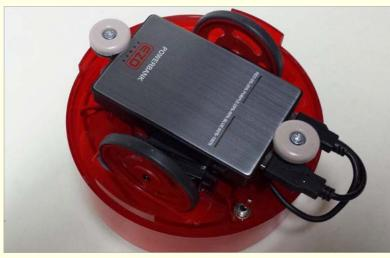
Above A standard smartphone battery pack is squeezed on top of the boards and inside the case
