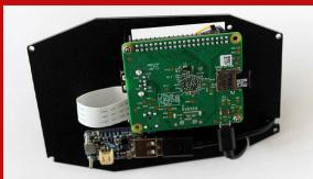
The camera case's customisable component holders are laser-cut from acrylic. "We've designed the inserts so that they perfectly fit all of the Raspberry Pi models currently available," explains Jon Fidler. "The design is very simple, using spacers, screws and nuts, making it accessible to anyone with a small screwdriver."
