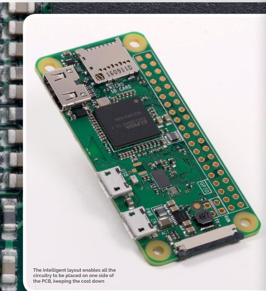
The intelligent layout enables all the circuitry to be placed on one side of the PCB, keeping the cost down
