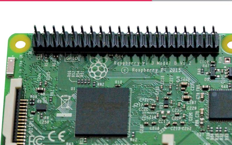
While it's possible to wire parts directly to the GPIO pins, most tinkerers place electronic components in a breadboard and connect this to the Raspberry Pi. Unlike the type used for cutting bread, an electronic breadboard is a plastic slab with lots of holes in it.
