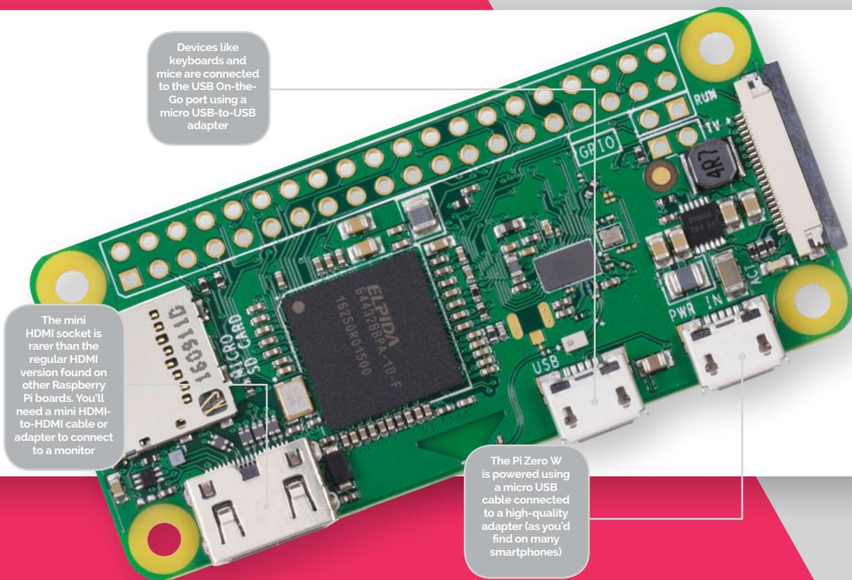
Devices like keyboards and mice are connected to the USB On-the-Go port using a micro USB-to-USB adapter
