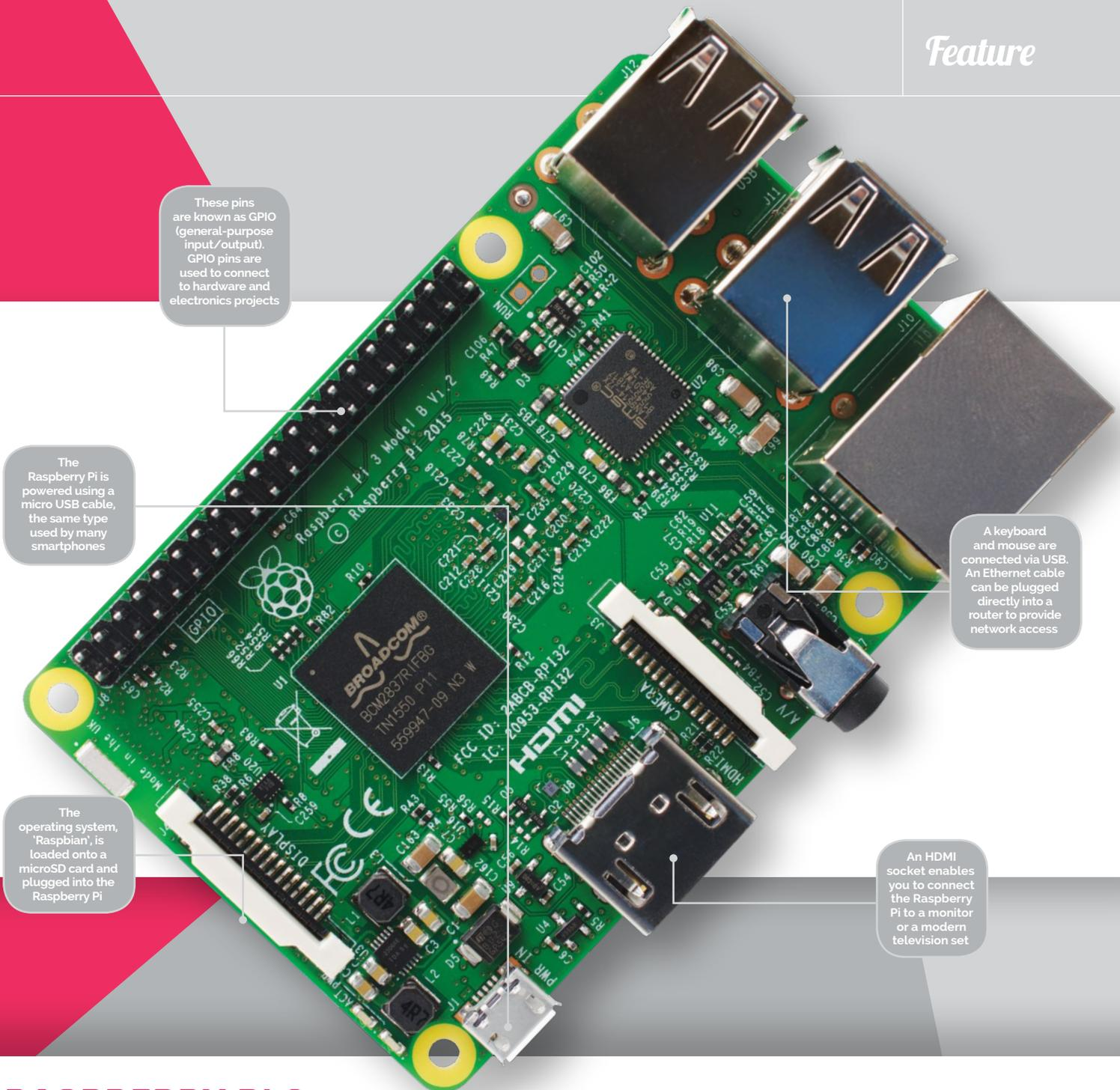
These pins are known as GPIO (general-purpose input/output). GPIO pins are used to connect to hardware and electronics projects
