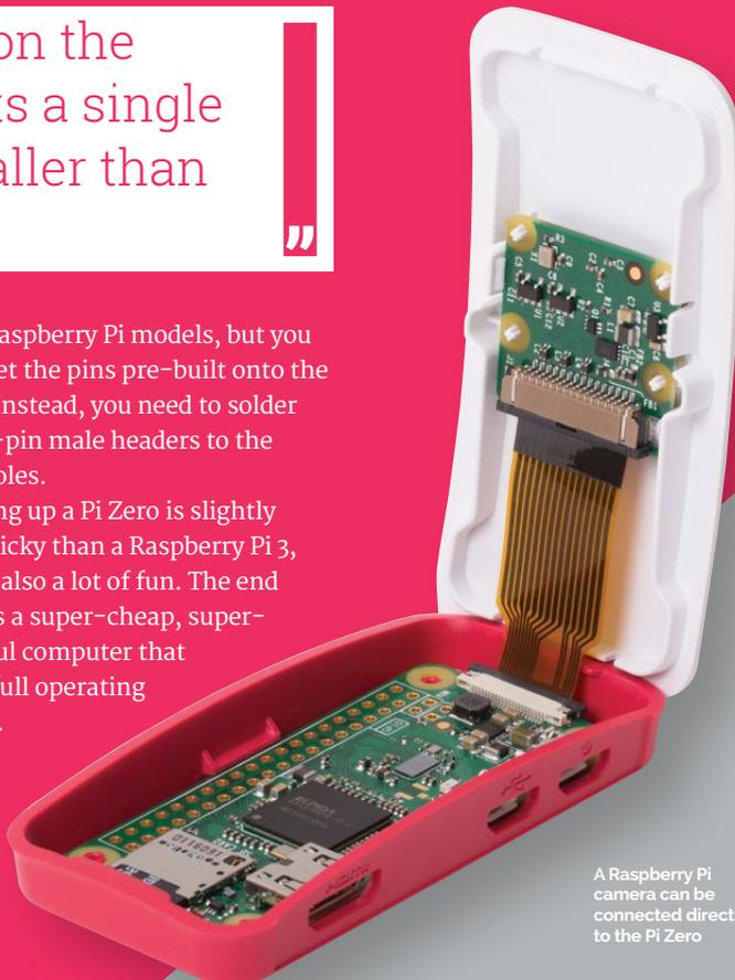
A Raspberry Pi camera can be connected directly to the Pi Zero
