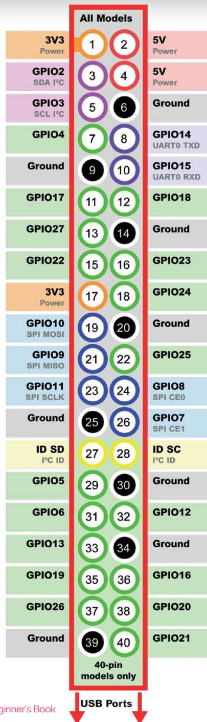
The 40 metal pins on your Raspberry Pi board are known as General Purpose Input/Output pins, or GPIO pins for short.
